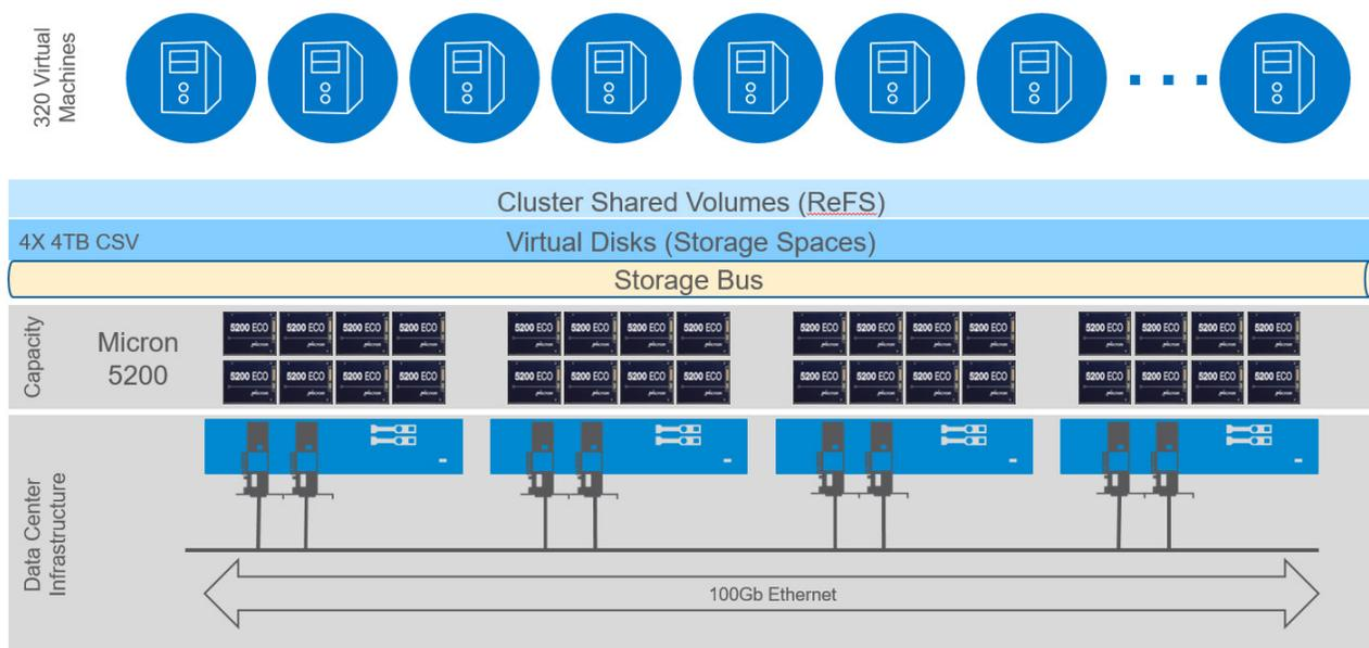
Figure 2: Micron's Hyper-Converged Infrastructure RA with Hyper-V and Storage Spaces Direct
