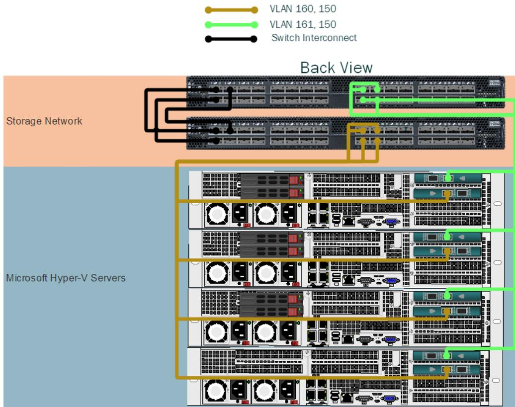
**Figure 3: Hyper-V/Storage Spaces Direct Cluster Physical Layout**
