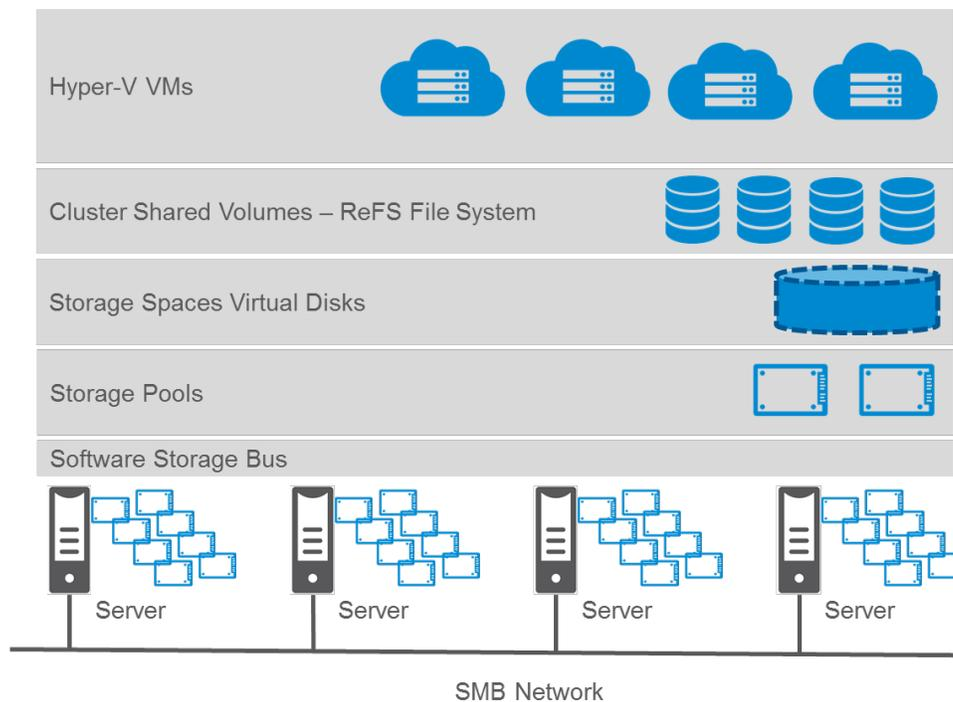
**Figure 1: Microsoft Hyper-V with Storage Spaces Direct Solution Overview**
