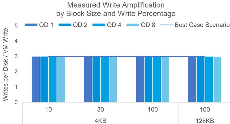
Figure 14: Write Amplification for Storage Spaces Direct
