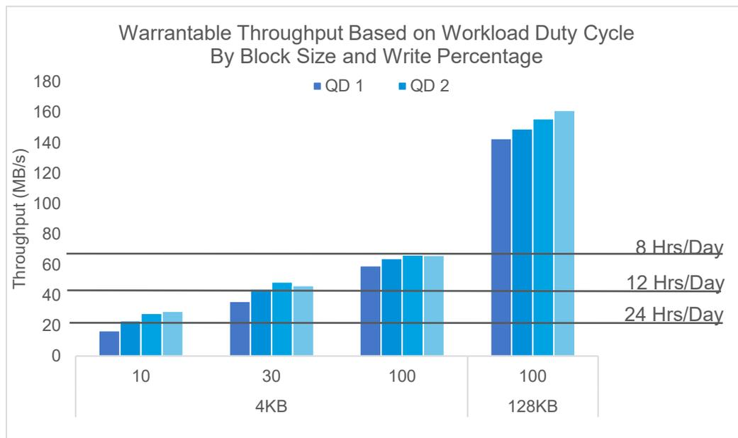
**Figure 12: Warrantable Throughput Based on Workload Duty Cycle**
