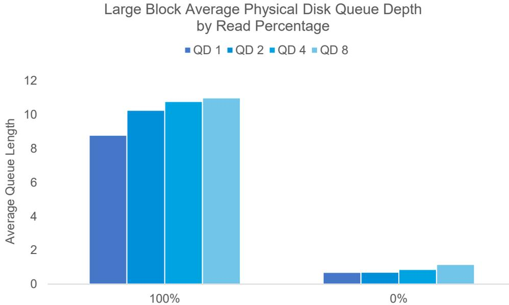
**Figure 11: Per SSD Queue Length for Large Block I/O**
