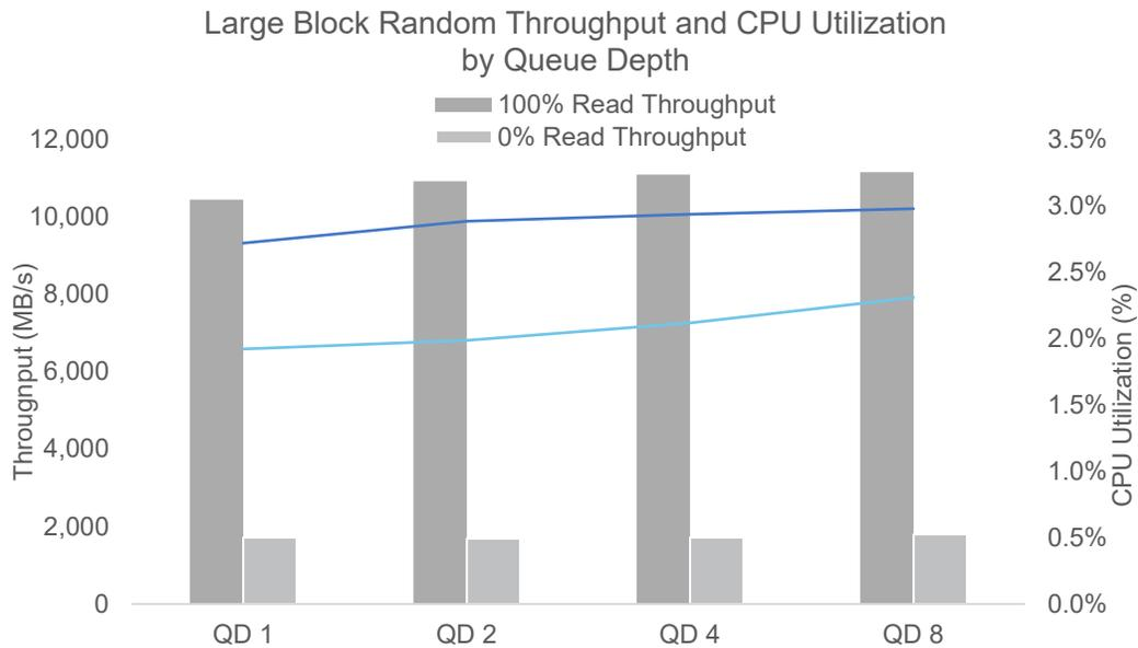
**Figure 9: Large Block Throughput and CPU Utilization**
